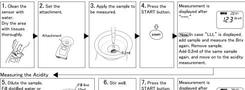
Memo A 1: 50 dilution can be prepared easily by filling the sample (stock-solution) to the line on the sample stage and filling water to the dilution line on the attachment
