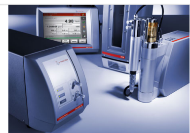
Turbidity Measuring Module: HazeQC ME
