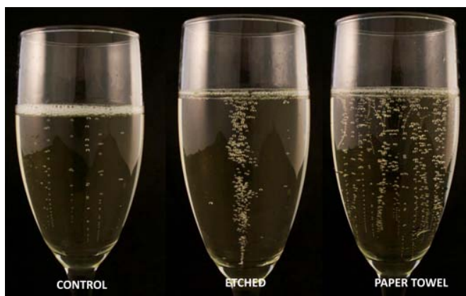
Figure 1 Picture of bubbles in sparkling wine glasses. Control: air dried, no etching; Etched: air dried, etched in base; Paper Towel: dried with paper towel, no etching.
