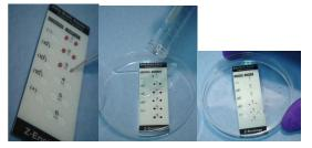
**STEP 3 – Anti-Brett Antibody** Sequentially add 5 drops **Anti-Brett (D)** and 5 drops of **Conjugate (F)** into the petri dish (beside the chip) containing Destain/Block. Mix by hand periodically (2 or 3 times) over 30 minutes.
