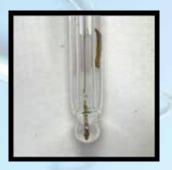
Never wipe the glass membrane because it can lead to permanent damage! DO NOT BE ALARMED IF ANY SALT DEPOSITS ARE PRESENT. This is normal with electrodes and they will disappear when rinsed with water.
