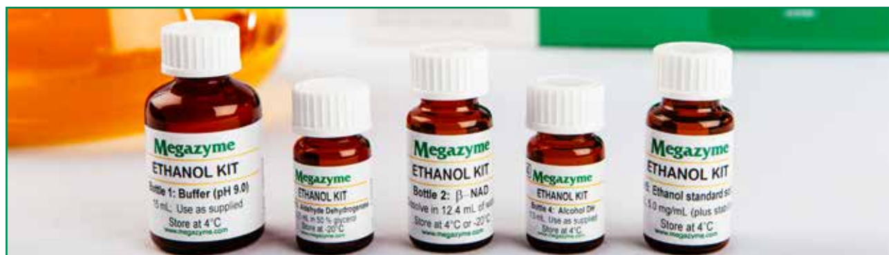
Figure 1. Left to right: buffer solution, reagent for first reaction, enzyme, cofactor for second reaction, standard solution.
