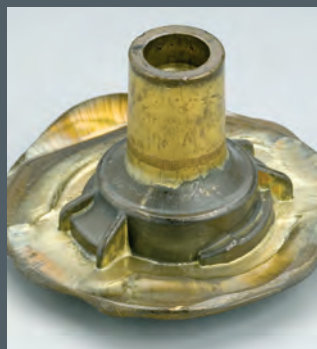
Forging of blank at approx. 700 °C
