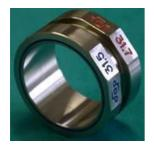
Place the ring, both sides successively, on top of the crown cap.
