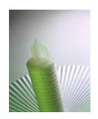
POLYSAN-PKP is obtained by pleating up to 5 polypropylene layers of decreasing porosity to achieve high effective filtration area, high dirt holding capacity and precise and controlled filter ratings. All the components in polypropylene are assembled by thermowelding process. POLYSAN-PKP is well suited in all applications (chemical—petrochemical—water treatment—food&beverage—RO—etc..) thanks to its
